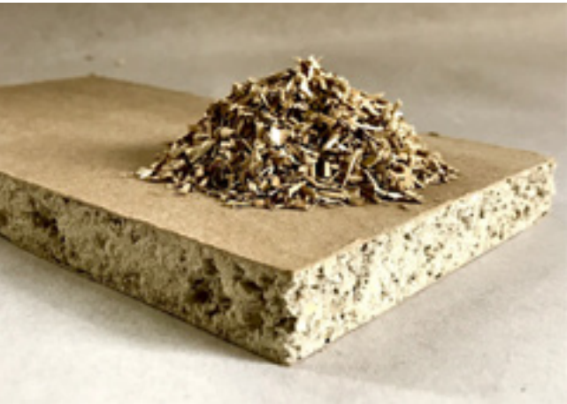
Biobased Lining Hemp and Lime board
